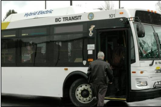
A BAE hybrid electric bus developed with NYSERDA support. Fuel savings exceed 25% from the HybriDrive® system and corresponding reductions in emissions of particulate matter, NOx and GHG are achieved. More than 4,000 hybrid buses now contain BAE's HybriDrive® system (over 40% of the total hybrid bus market) comprising the largest fleets in New York City, London and elsewhere.
